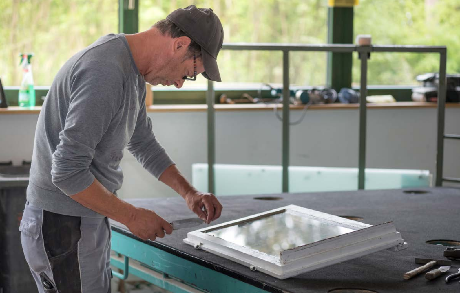
A glazier working on an energy-efficient, triple-gazed window.
